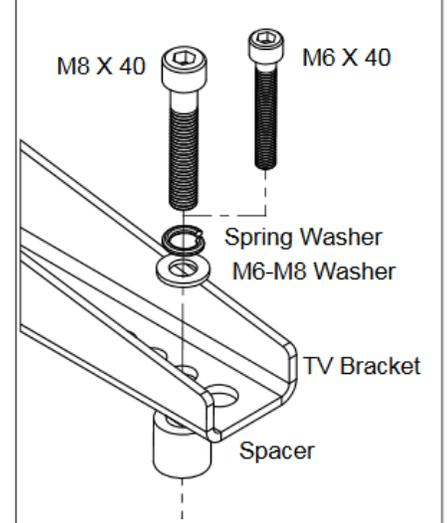
Spacer is used when the back of TV is not flat or the mount holes are sunk into the back of the TV. (Rarely used)
