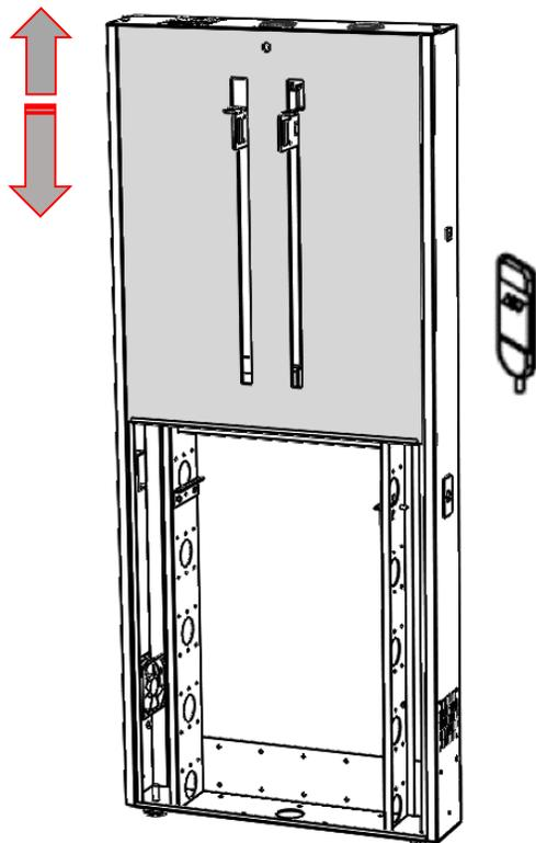
**7** Insert Tube into carriage openings.
